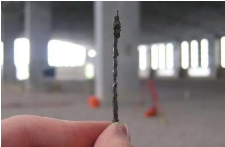
Figure 17. Metallic fibers for concrete reinforcement
